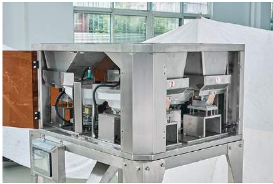
Details of K3-100 Suger Sachet Packing Machine
